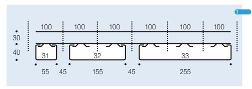
Installed in the same modular carrier all types have an open gap of 45 mm.
