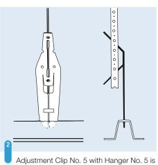
located into the slots provided in the modular carrier.
