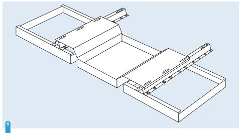
The downlight adapter is available in 300 mm modular size and supplied in any colour for direct integration into the DAMPA $^{\circ}$  Interval system.
