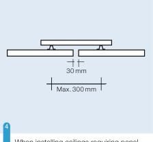
When installing ceilings requiring panel lengths greater than 6 m, jointing can be achieved by forming a desired gap between the ends of the panels.
