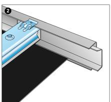
It may be necessary to provide additional support in close proximity to other integrated components, e.g. lighting and ventilation, to avoid excessive ceiling deflection.
