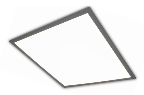
LED Clip-in Panel fits DAMPA® Clip-in Tiles High quality LED chip 0.2W/pcs. Panel dimensions: 300x300, 600x600 mm Lifespan: >50.000 hours.
