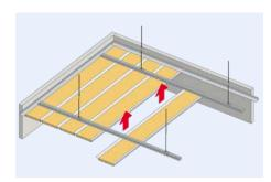
The DAMPA® DCC 300/200 Ceiling Panels are normally installed progressively, starting at either end of the room. However, panels can be left out at any position to be installed later.
