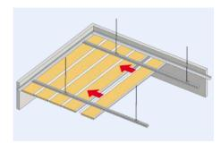
After aligning the leading and returned flanges with the clips of the modular carriers, the panels are engaged starting at one end.
