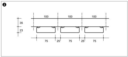
2 A 100 mm module is obtained with 75 mm units and an open gap of 25 mm.
