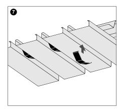
When installing ceilings requiring panel lengths greater than 6 m, jointing can be achieved by forming a gap of 10 to 25 mm between the ends of the panels immediately
